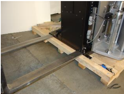
Using forklift from rear of machine place forks in upper half of channel frame.
