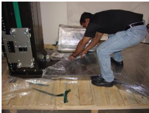
Push tower upward into up right position.
