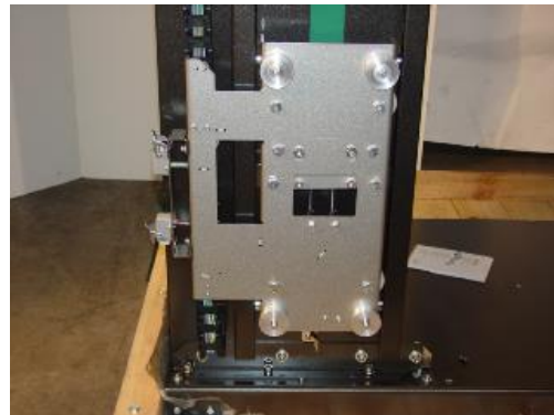
* Note-The pre-stretch unit is extremely heavy. Use two people to lift into position.
