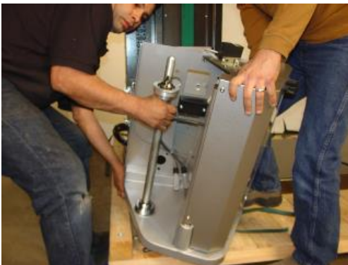
* Note-The pre-stretch unit is extremely heavy. Use two people to lift into position.
