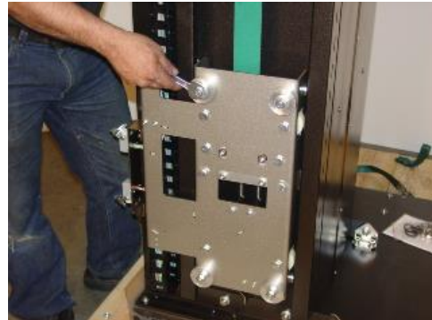
Remove 4 nuts and washers from pre-stretch mounting plate.
