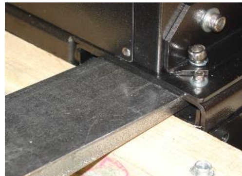
Using forklift from rear of machine place forks in upper half of channel frame.
