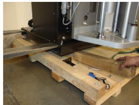
Insert 2X4 underneath frame to raise up
